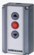
Push button DTH R For separate control of both operational directions, with separate stop button. Protection category: IP 65 Dimensions: 90 × 160 × 55 mm (W × H × D)
